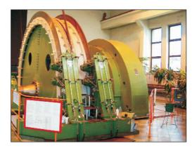
The sensors signal possible deviation of the disk or its segment. Moreover, every disk is fitted with an infrared sensor, which checks possible overheating of the disk over the permissible limit. The main shafts are manufactured as shaped, with connectable flanges. For rotor placement we use flange connection, or more often the rotor is placed directly on the main shaft.
