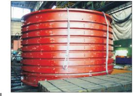
The segments are screwed to thickened side plates of disks using the analogous technology as that used with connecting frictional disk halves (hydraulically tightened screws with defined axial pre-stress). Mutual location of individual segments is stabilized by the help of locks of groove and tongue type. To every brake disk, sensors automatically checking the extent of its axial run-out are installed on mounting.
